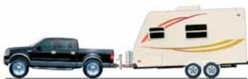
Using a weight-carrying hitch
